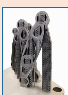
Optimized suspension arms printed according to two different orientations to investigate the differences introduces by dissimilar surface direction and supports position.
