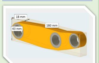
To perform optimization of the part, the geometry is divided in the "design space" where material is present but can be removed to optimal achieve an geometry, and the "nondesign space", where material and geometry are fixed to guarantee necessary interfaces (bearing seats etc.), that define boundary conditions
