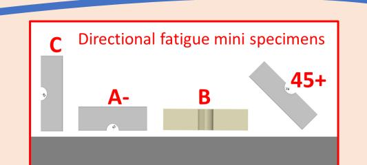
Miniaturized specimens divided into four different orientations produced to evaluate effect of build direction on fatigue performance of the material and to generate fatigue data useful for the part qualification phase.
