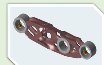
Topological optimization based on SIMP-algorithm (solid isostatic material with penalization) that attributes a varying density to each element. The optimization goal is defined in terms of minimization of the mass and global maximization of the stiffness. The solution respects imposed limits and is characterized by the best stiffness-to-weight ratio.
