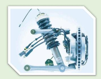
The identified component is the lower suspension arm of a car which develops a key structural function as it is connected to the chassis, to the wheel upright and the shock absorber. The scaled version of the suspension arm was selected because it is subjected to dynamic loading and therefore it requires a fatigue integrity assessment at design stage and experimental subsequent verification.
